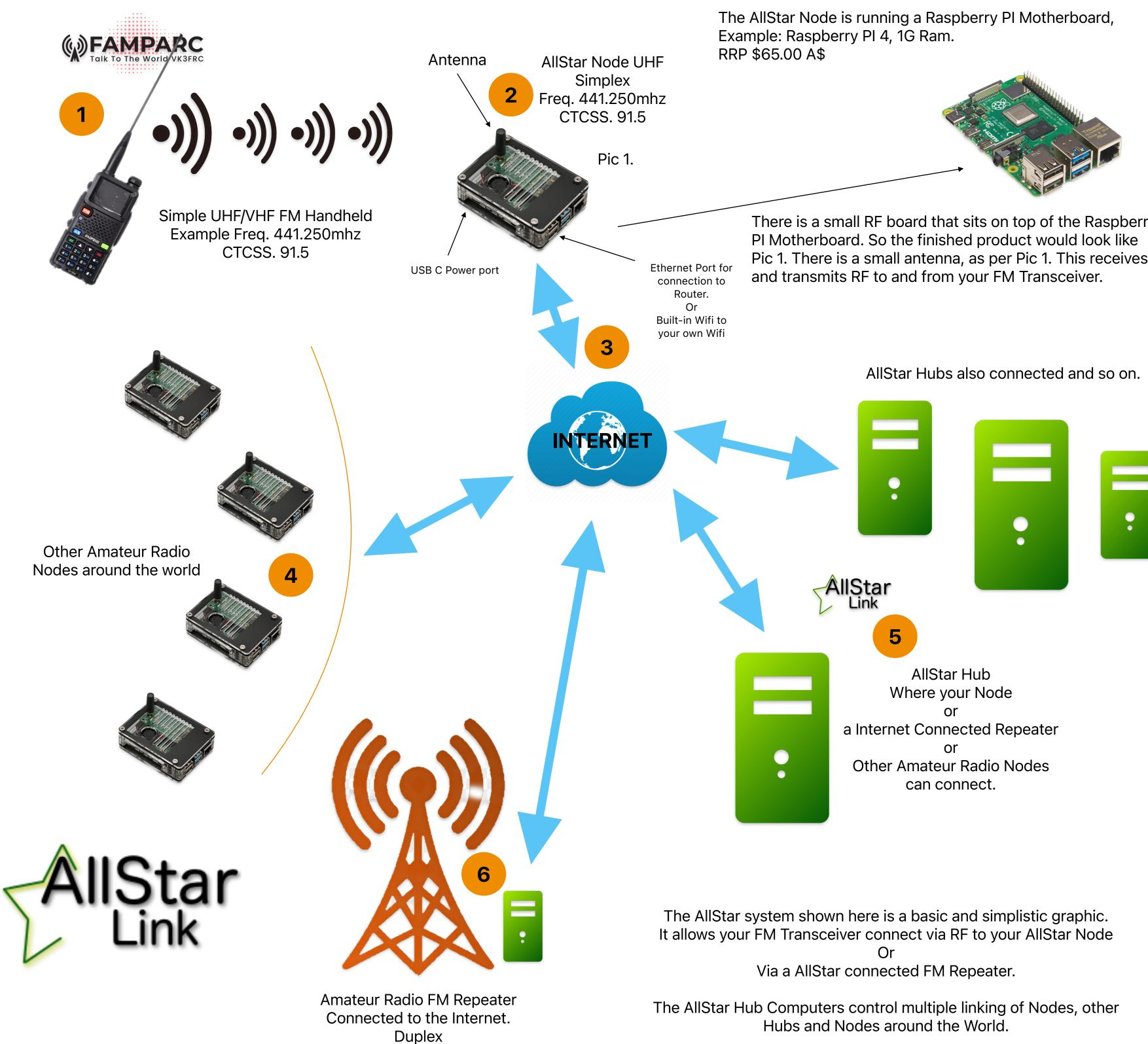
There is a small RF board that sits on top of the Raspberry Pic 1. There is a small antenna, as per Pic 1. This receives
