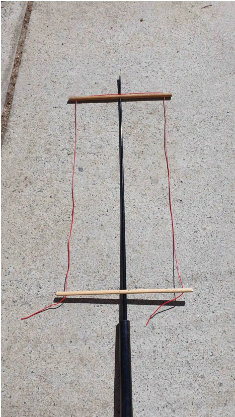
145 MHz Rectangular Loop Antenna layout 360 mm x 690 mm
