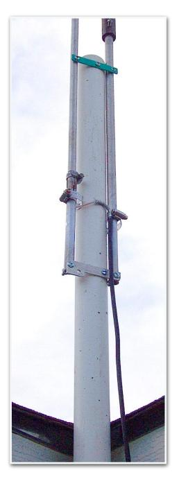
I found that the Slim Jim could bring up several repeaters that the J Pole could not! No changes were made between the two comparisons except the antennas!
