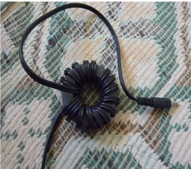
Twin shielded speaker cable wound on T200 toroid
